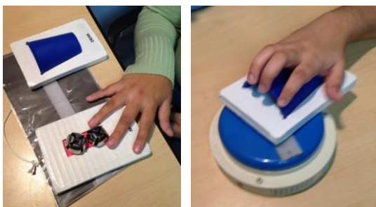
STACS symbols (APH) used on a choice board and a 1-cell voice output switch.
